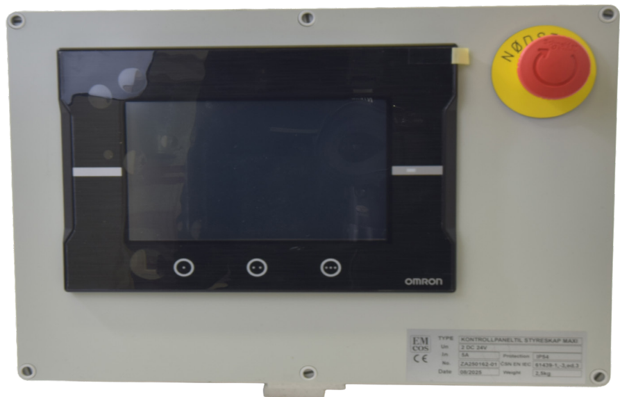
Figure 18 Control box with screen and emergency stop button
