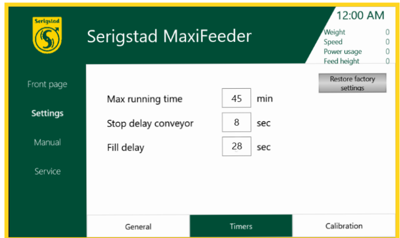
Figure 21 Screenshot of settings - timers - numbers are examples, and not the factory settings
