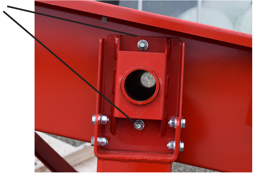
Figure 13 Mounting the stand to the base frame.
