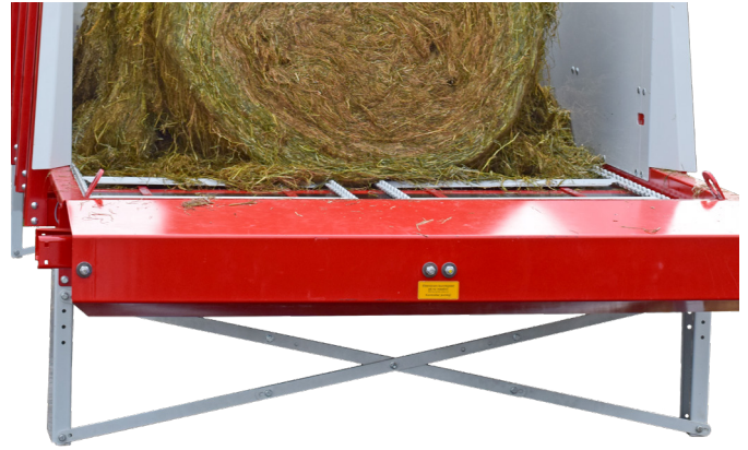
Figure 8 Installed standard leg set.
