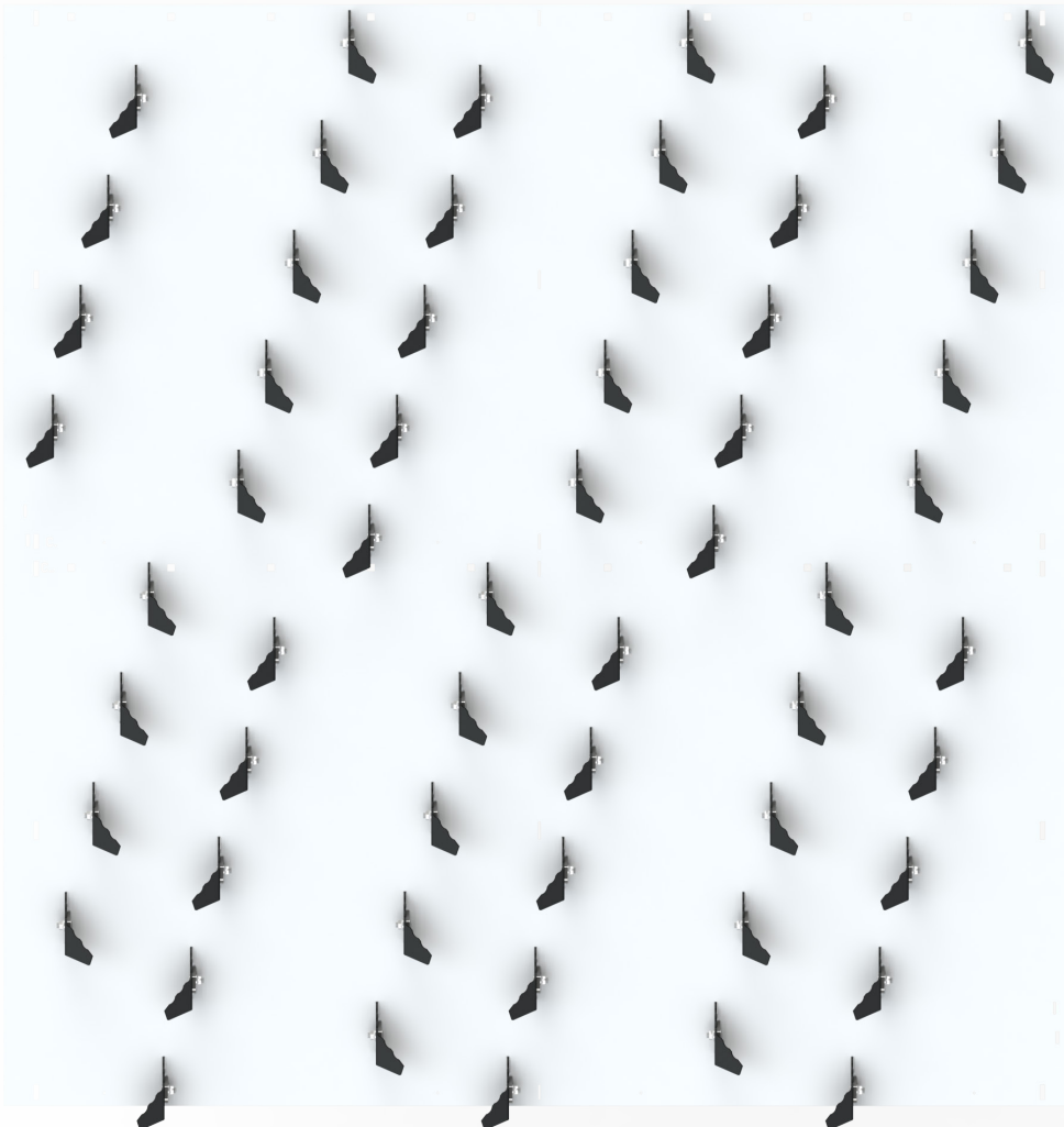
Figure 26 “Unfolded” knife drum with the standard knife configuration of 58 knives. This distribution ensures smooth and balanced operation of the knife drum.
