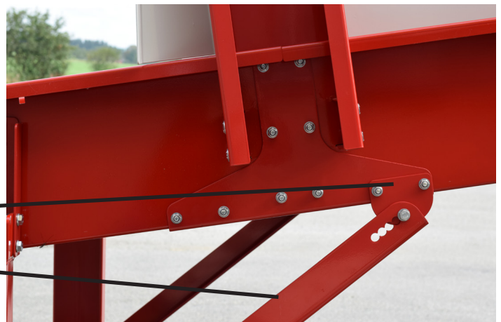
Figure 12 Bracing rod connected to the base frame with the bracket.
