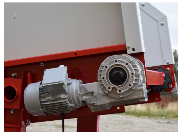
Figure 40 Motor and gearbox for conveyor belt.
