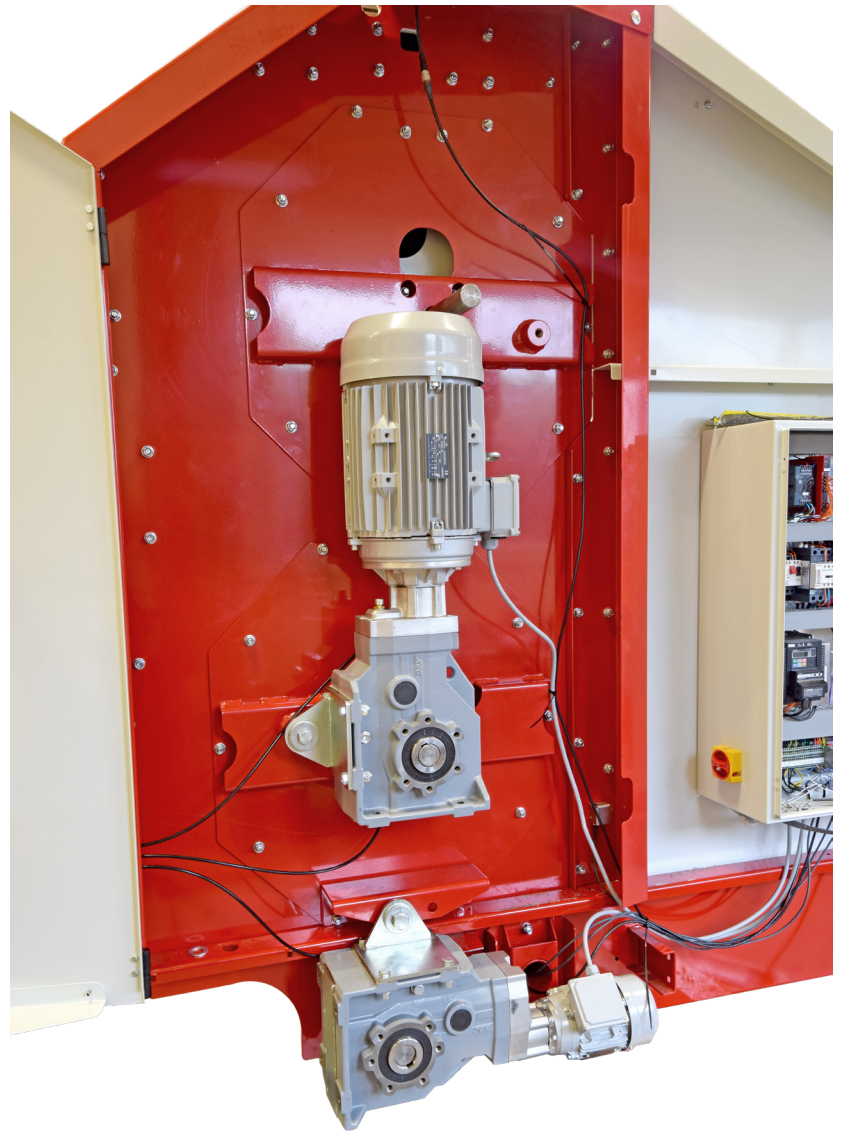
Figure 19 Motor and gearbox for the knife drum and conveyor belt
